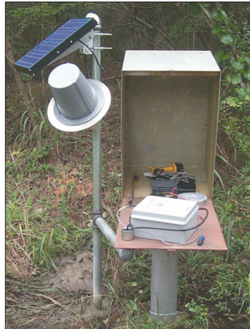
Figure 2. A, Data logger and incremental encoder. B, Integrated data logger/encoder. C, Data logger, encoder, and satellite-transmission equipment. Brand names are for illustration purposes only and do not imply endorsement by the U.S. Geological Survey. (Photographs by W.L. Cunningham.)
